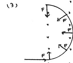
(4) The magnetic force is always at  $90^\circ$  to the velocity of the proton  $\therefore$  it moves in a circle if the force is a centripetal force.
