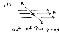
11. Vector addition of the permanent magnetic field  $B$  and that generated by the current in the wire.
