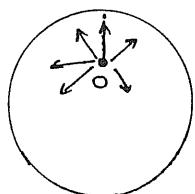
As an object o moves below the surface, mass above it attracts it in the opposite direction to the mass below it.  $\therefore$  The resultant force is less.  $\therefore$  less  $g$ .
