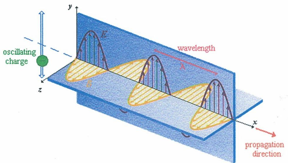
1. When a changing potential difference is applied to a conductor the electrons experience a force which causes them to accelerate
