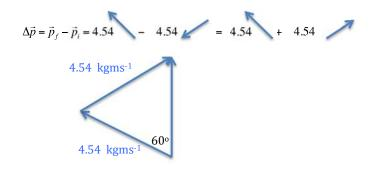
As can be seen by the vector triangle above,  $\Delta \vec{p}_{\text{ball}}$  is directed 90° away from the wall .
