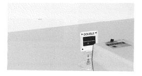
The distance between the slits is  $6.5 \times 10^{-5}\,m$  and the slit-to-screen distance is  $0.42\,m.$  The student measures the distance between two adjacent maxima at the centre of the interference pattern on the screen as  $4.0\,mm.$
