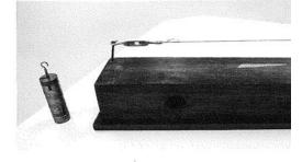
Students conduct an experiment, using a sonometer. The tension in the wire is varied by increasing the mass that is suspended from one end of the wire. The lowest frequency of the vibrating wire is measured (in hertz), using an appropriate app (application) on a smartphone, as shown in the photograph on the right.
